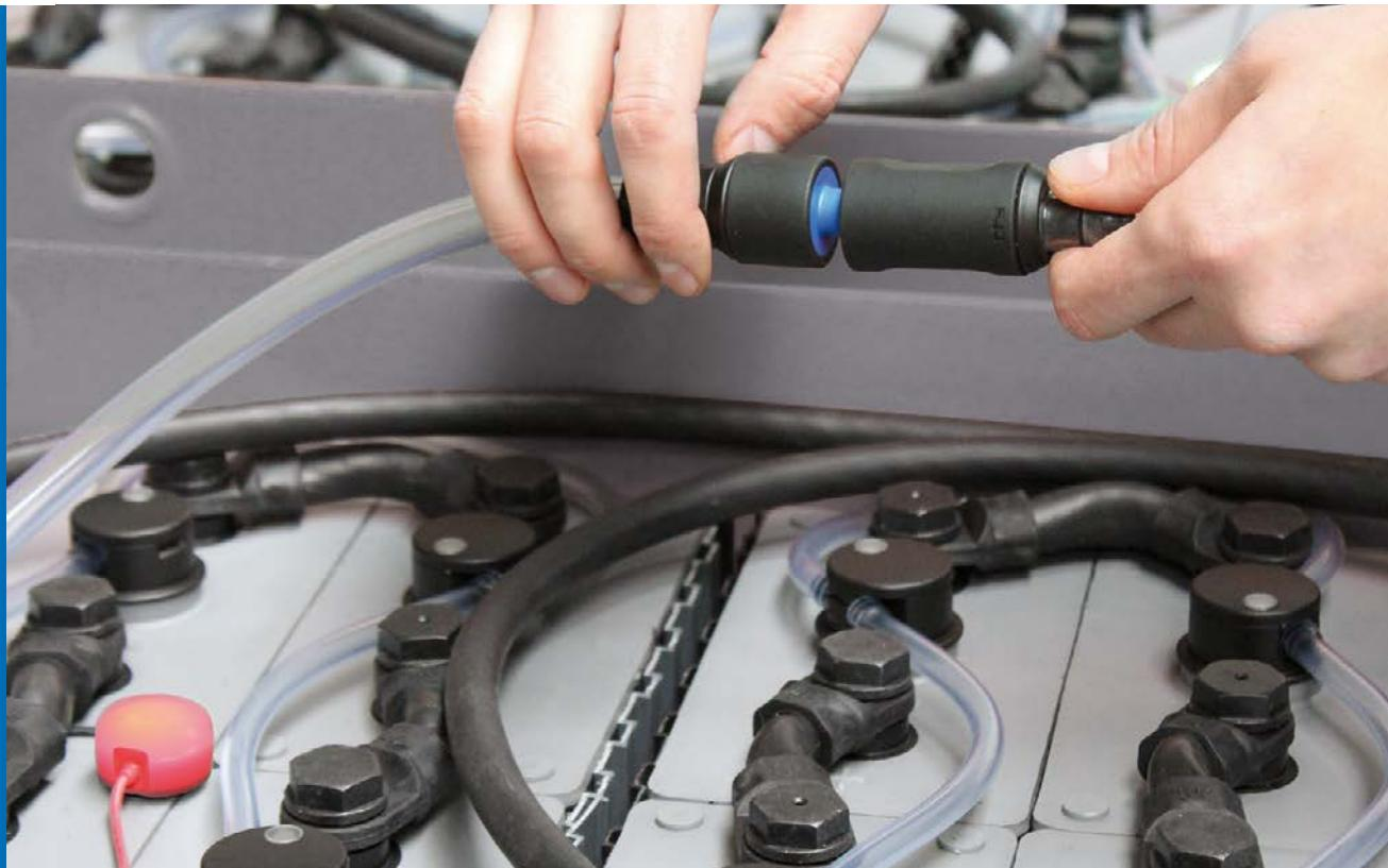
One of the most important components for the function of traction batteries with lead-acid technology is the electrolyte; a solution of sulfuric acid and water. When batteries are recharged, water is converted into hydrogen and oxygen by electrolysis. This water consumption must be compensated with demineralized water shortly before the end of charging in the case of batteries with liquid electrolyte. High requirements apply to the purity of the refill water.
